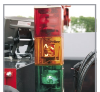
Overload warning lamps + auto stop + alarm
